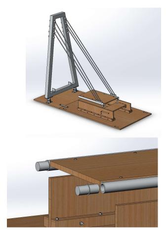
4. Install panel A with its cables. Make sure you use the single coloured cables for this side of the pier. The lugs and the end of each cable is colour coded.
