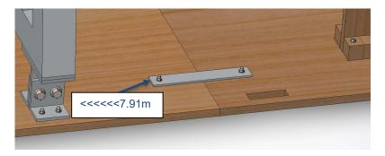
2. Install panel A as shown and connect the cables for panel A. NOTE – All panels are colour coded with electrical tape. You need to match the colours. We have single colours and double colours. Single colurs are on the step side (outer most side) and the doubles run towards the middle. The same applies for the cables which are also colour coded. These will need to be prehung for the smaller children.
