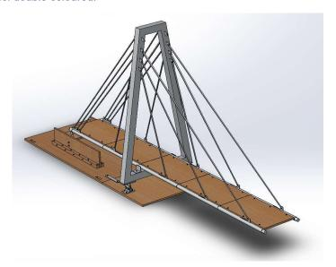
6. When you get to panel E install the sliding bolt ready to slide into panel E1. NOTE – You will need to install panel E1 before panel E due to the steel plate that panel E will rest on.
