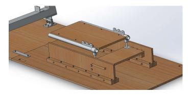
3. Connection pins are installed on the end of panel A
