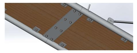
8. Extend the sliding boss. Finally, you may need to adjust the turn buckles to have a little slack (we need some slack for when the students/teachers walk over it – one at a time – although you can have several technically). There will be significant adjustment required when on an unevan surface/slight slope).
