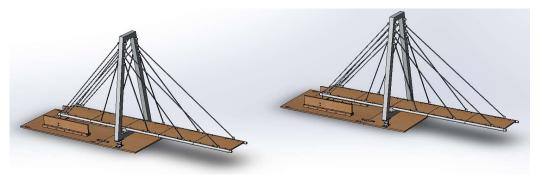
7. Connect the panel E and E1 by steel panel and M8 bolts. Nuts facing down, sockets are drilled to hide the bolt heads.
