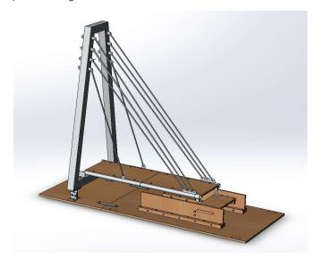
5. Repeat the process with panel B as shown and so for the rest of the panels. There should be 5 No. panels each side in total (panels for other side of the birdge are A1, B1, C1, D1 and E1). The panels on the other side of the pier running towards the middlel double coloured.
